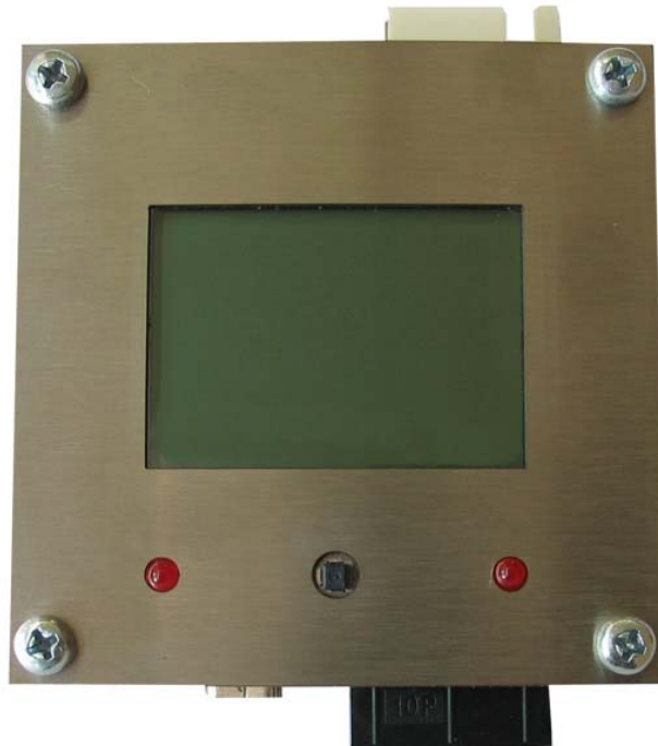
Figure 17. Above is the Olimex PIC-LCD3310 development board used as the remote device in this project. [39]
