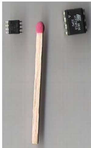
Figure 15. This image shows two Atmel ATtiny13 microcontrollers. On the left is the device shown in the Small-Outline Integrated Circuit (SOIC) package, and in the Plastic Dual In-line Package (PDIP) on the right. [37]
