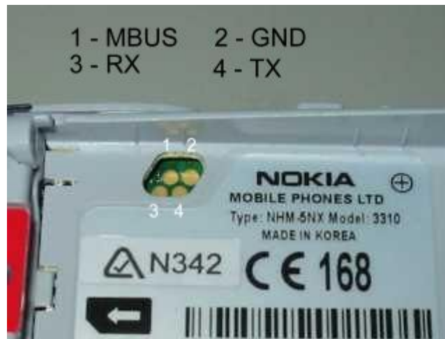
Figure 20. The Nokia F-Bus and M-Bus contact pads are shown above. [23]
