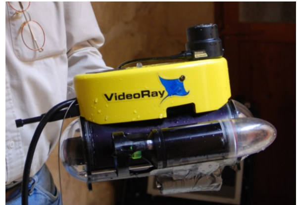
Figure 1: The VideoRay Pro III ROV. In this image, the supporting feet of the ROV have been removed to allow entry through the smallest cistern passage. The cistern was located in a private home of the Mdina fortress.
